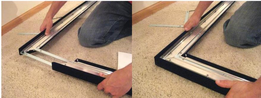
**Ball-Point Wrench the Set Screws.** Confirm with your fingers at the joint that they are perfectly joined and then start tightening the set screws. Use the ball-point end of the wrench provided so that you can more easily access the screws and won't over tighten them. Repeat this so that you've joined the top, bottom and one side piece, saving the other side piece for last.
