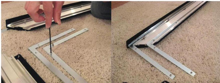
**Install L-brackets.** Align the L-brackets into their mating slots in the other frame member, and slide them together making a nice tight corner
